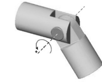
Fig. 30. Revolute joint: one degree of freedom.
